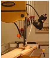
We built-in a handy work light on a flexible shaft to make seeing what you are doing a little easier.
